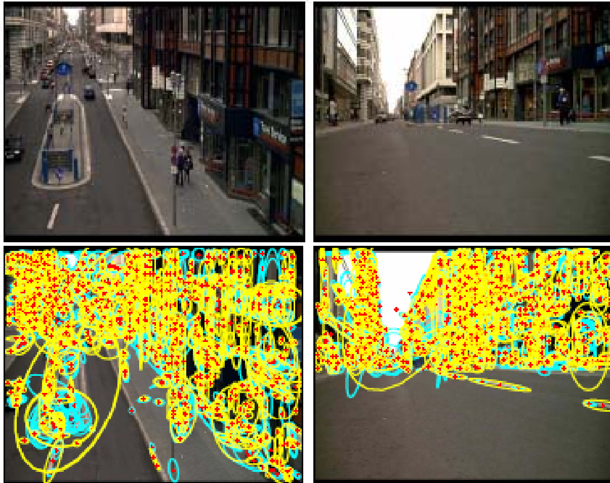
Figure 1: Top row: Two frames showing the same scene from very different camera viewpoints (from the film 'Run Lola Run'). Middle row: frames with detected affine invariant regions superimposed. 'Maximally Stable' (MS) regions are in yellow. 'Shape Adapted' (SA) regions are in cyan. Bottom row: Final matched
